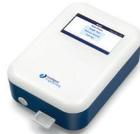
Analyses the Drug Screening Cartridge to provide clear on-screen results in 10 minutes.
