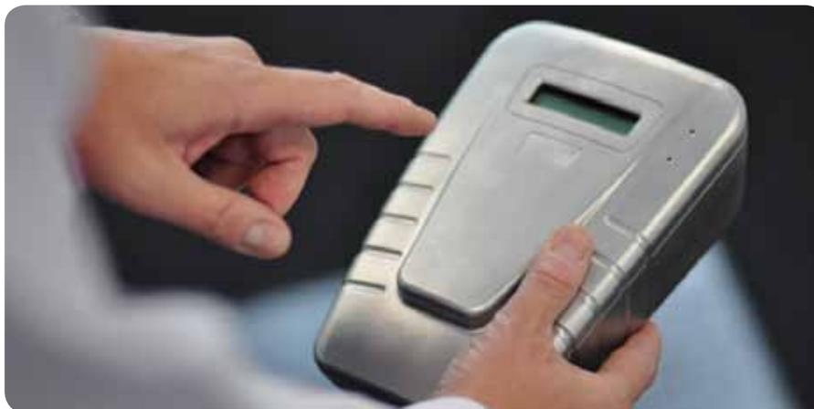
Prototype of the Intelligent Fingerprinting hand-held sample collection and analysis device. The use of this device will allow samples to be collected from individuals' in-situ, with results available from analysis using disposable analysis cartridges in a matter of minutes.
